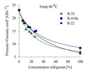
*Figure 6 Predicted pressure-viscosity coefficient vs. concentration.*
