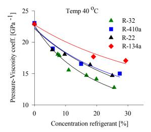
*Figur 4 Pressure-Viscosity coefficient vs. concentration at 40°C.*
