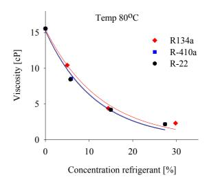
Figure 3 Viscosity vs. concentration at 80°C.
