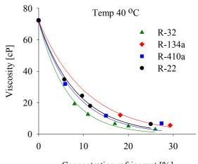
Concentration refrigerant [%] Figure 2 Viscosity vs. concentration 40°C.
